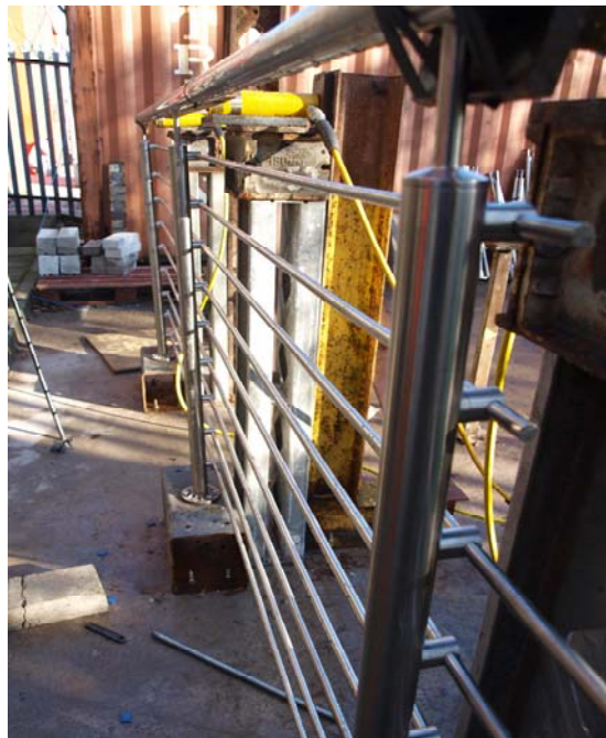
Photograph 4: Load being applied to the handrail of balustrade test system 6.
