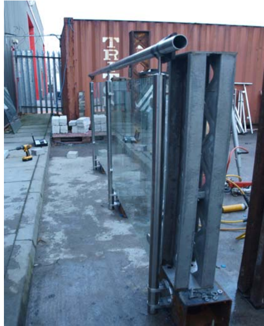
Photograph 5: Testing of side mounted balustrade fixing.
