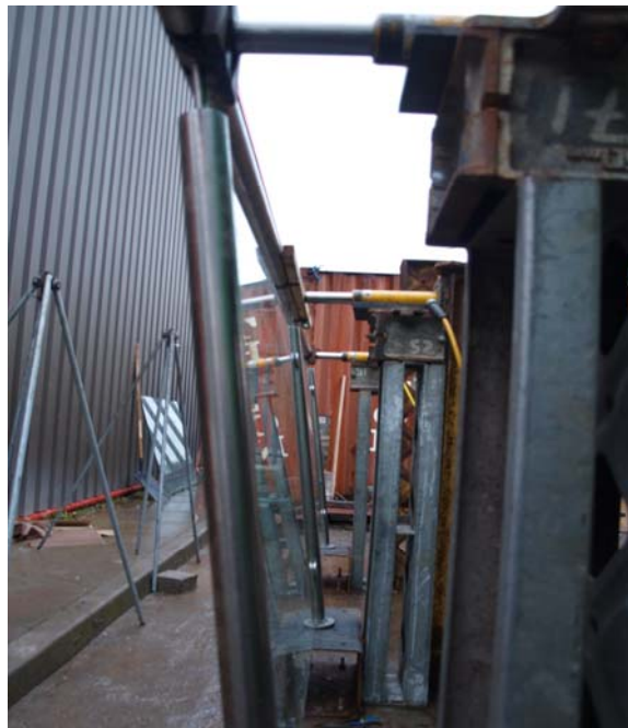
Photograph 8: Testing balustrade system beyond acceptable limits.
